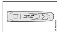
Your saw comes standard with a chain scabbard that matches the cutting attachment.
