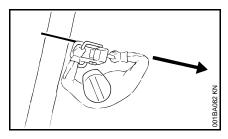
Position the saw so that your body is clear of the cutting attachment.
