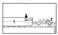
Lay the appropriate file gauge (1) for the chain pitch on the saw chain and press it against the cutter to be checked – if the depth gauge protrudes past the file gauge, the depth gauge must be reworked Saw chains with humped drive link (2) – upper part of the humped drive link (2) (with service mark) is lowered at the same time as the depth gauge of the cutter.
