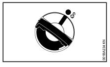
Marks on tank cap and fuel tank must line up.
