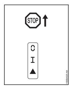
STOP or 0 – Master Control lever must be pushed in direction of STOP or 0 to switch off ignition. The Master Control lever springs back to the run position I when it is released.
