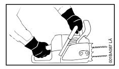
Always hold the chain saw **firmly with both hands:** Right hand on the rear handle – even if you are left-handed. To ensure reliable control, wrap your thumbs tightly around the handlebar and handle.
