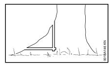
Make the vertical cut first, then the horizontal – but only if the wood is sound
