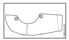
Under extreme winter conditions (temperatures below -10 °C, powdered or drifting snow), it is recommended to mount the cover plate (special accessory) on the fan housing.
