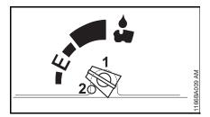
The oil flow can be adjusted as needed using the adjusting screw (1) (on the bottom of the machine).
