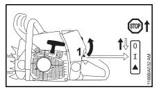
Move the Master Control lever in the direction of STOP or 3 – when released, the Master Control lever springs back to the normal run position I.
