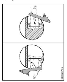
Perform this felling cut when the tree diameter is greater than the length of the guide bar.
