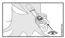
Use the plunge-cutting sight if possible. The plunge-cutting sight and the top and bottom of the guide bar are parallel.
