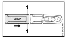
Push the scabbard extension and chain scabbard together – the lugs (1) must engage in the chain scabbard.
