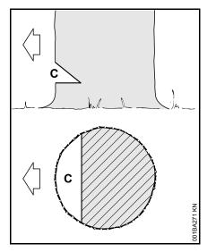
The felling notch (C) determines the direction of fall.
