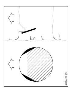
Sapwood cuts in long-fibered softwood help prevent sapwood splintering when the tree falls. Make cuts at both sides of the trunk at same height as bottom of felling notch to a depth of about 1/10 of trunk diameter. On large diameter trees, cut to no more than width of guide bar.
